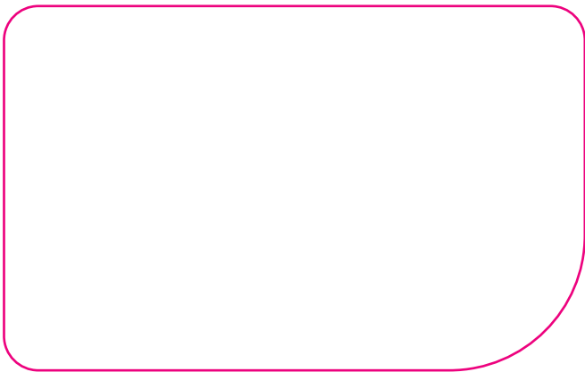
2M_86x54mm_Multiple rounded corners 86x54mm with 5mm rounded corners x3 20mm rounded corner x1
