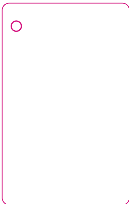
2M_54x86mm Tag 54x86mm with 3mm rounded corners 2mm diecut hole
